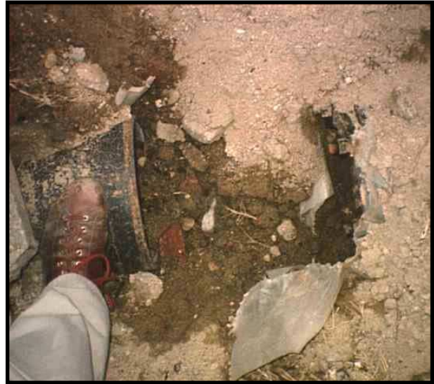
Photos 1A and 1B showing ground cracking due to liquefaction/lateral spreading in the vicinity of Osaka Bay, and a pulled joint in a ductile iron pipeline (Kobe 1995).
