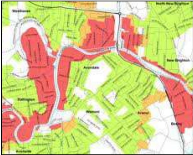
Figure 4. Extreme liquefaction (in red) along the Avon River in Christchurch New Zealand.
